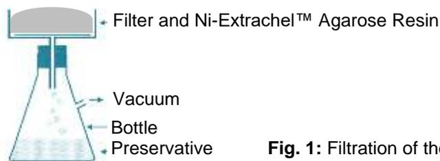
**Fig. 1:** Filtration of the Agarose suspension
