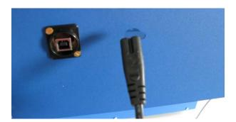
8. Connect the power cable with the power adaptor and the USB cable with the USB connection of the cabinet. Switch on the camera. Close the drawer and screw it tight.
