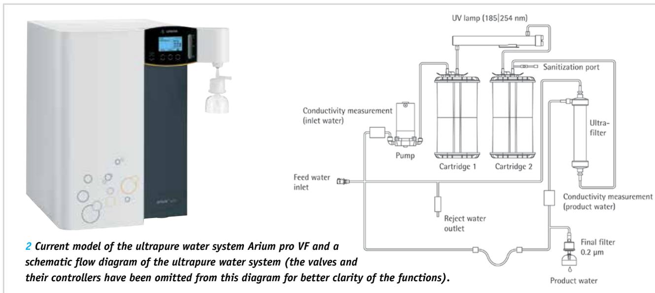
**2** Current model of the ultrapure water system Arium pro VF and a schematic flow diagram of the ultrapure water system (the valves and their controllers have been omitted from this diagram for better clarity of the functions).
