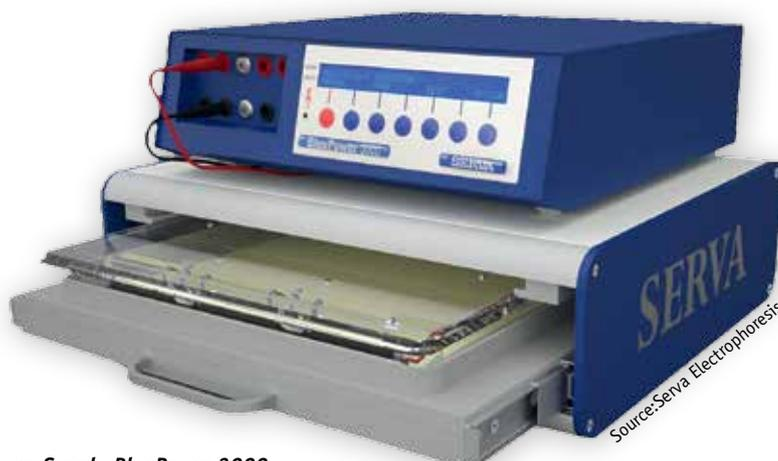
**3** Hofer Inc. IEF100 (a) and HPE BlueHorizon (b) with Power Supply BluePower 3000
