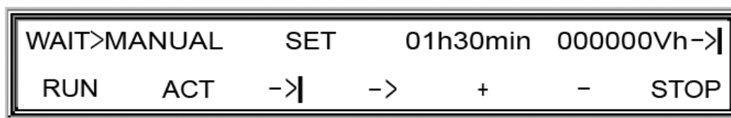
Fig. 12: Display of the preset limits of the break off parameters MANUAL-[WAIT]
