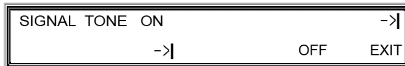
Fig. 36: Display of the OPTION signal tone: ON
