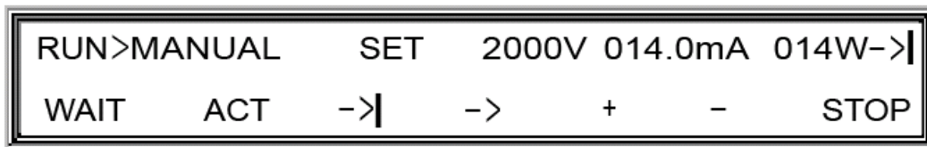
Fig. 8: Display of the preset limits of the electrical parameters MANUAL-[RUN]
